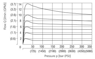
The characteristic of the pressure compensator corresponds to the flow rate of a PRM2-043Z11/12 proportional directional valve.
